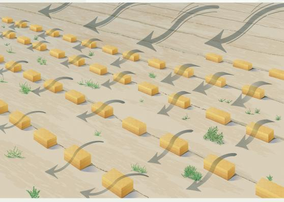
Bales reduce wind speed and dust emission and provide conditions for plant survival and growth.
